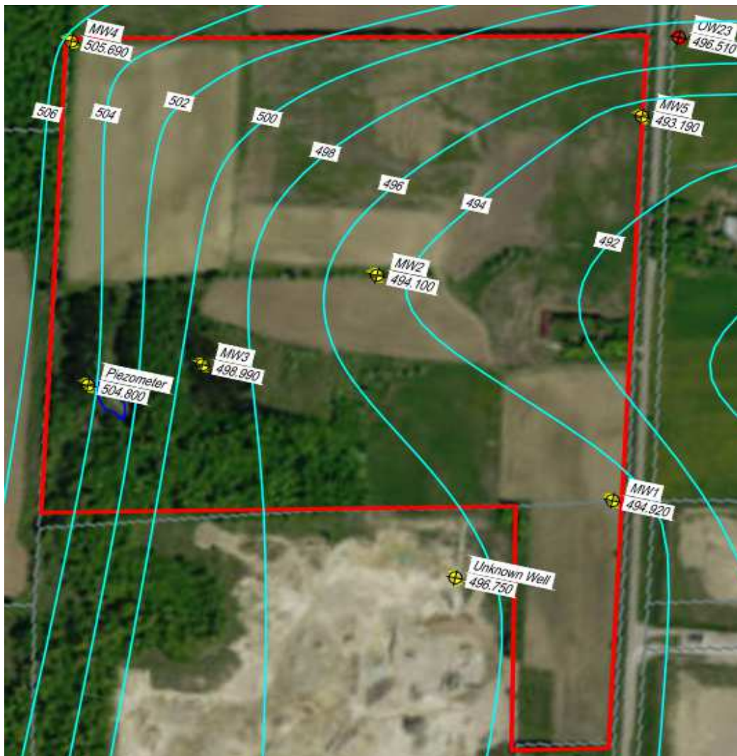
Figure 12: Local Ground Water Contours
