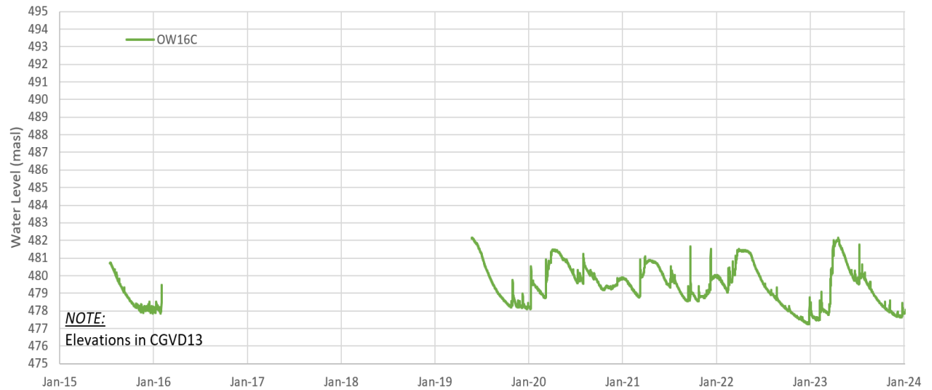
Figure B.16: Hydrograph of water levels at Well OW16C, in masl.
