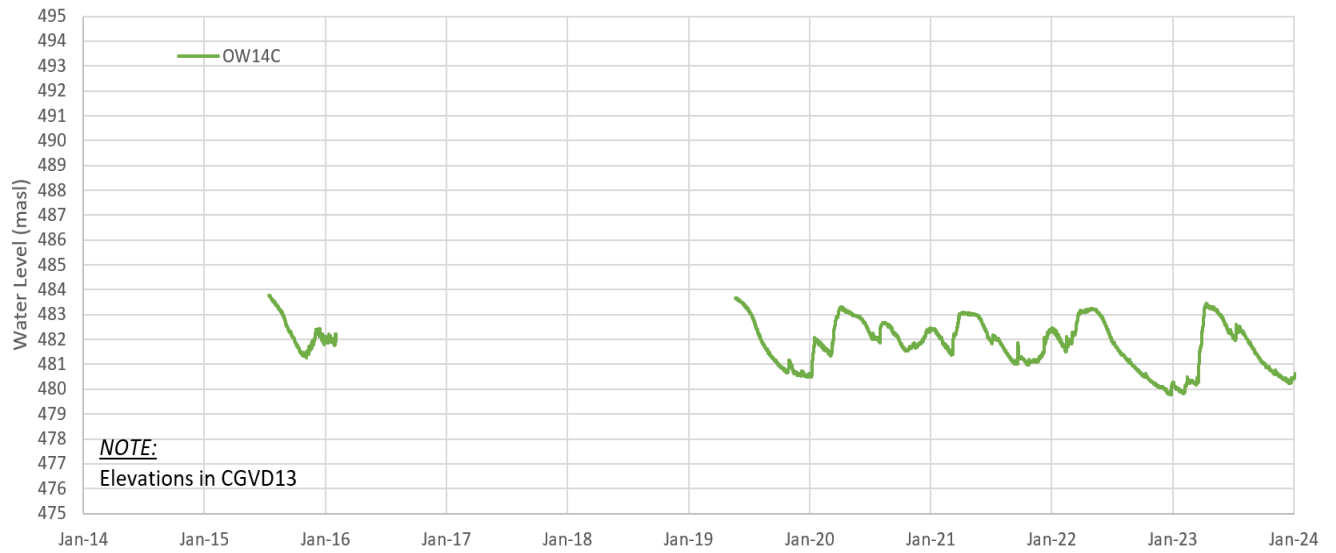
Figure B.15: Hydrograph of water levels at Well OW14C, in masl.
