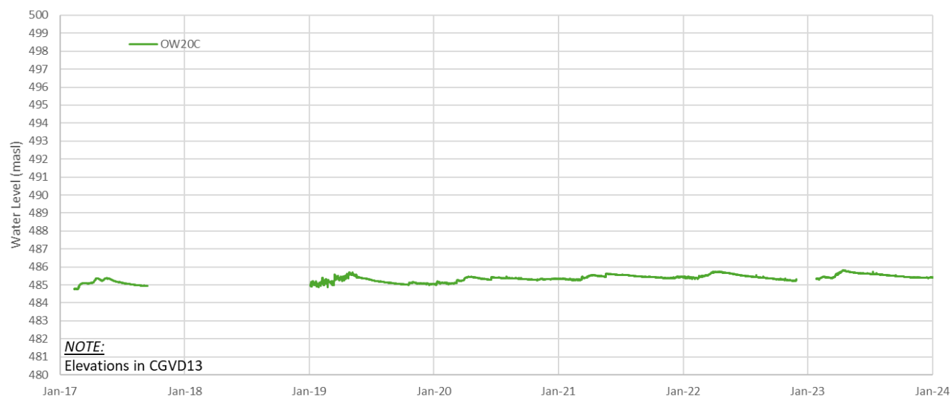
Figure B.21: Hydrograph of water levels at Well Nest OW20C, in masl.
