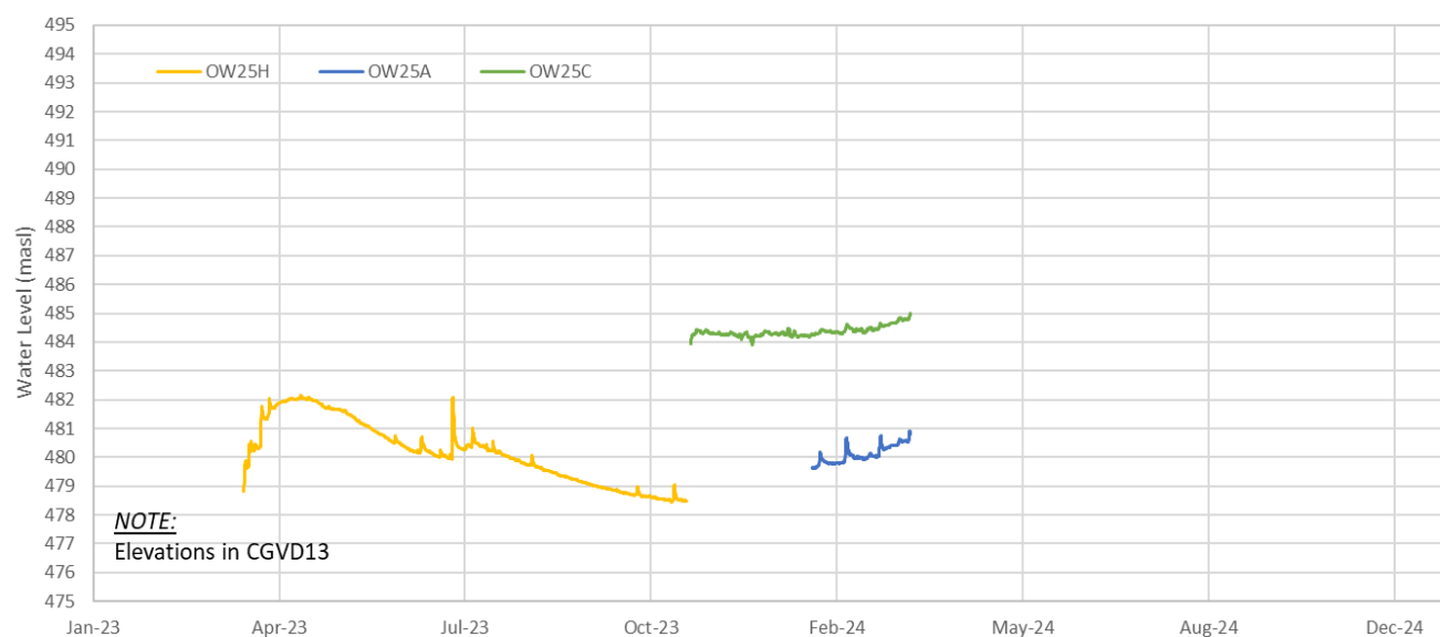
Figure B.25: Hydrograph of water levels at Well Nest OW25, in masl.
