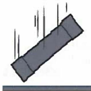
FREE DROP A 9-metre (30-foot) free-fall onto an unyielding surface
