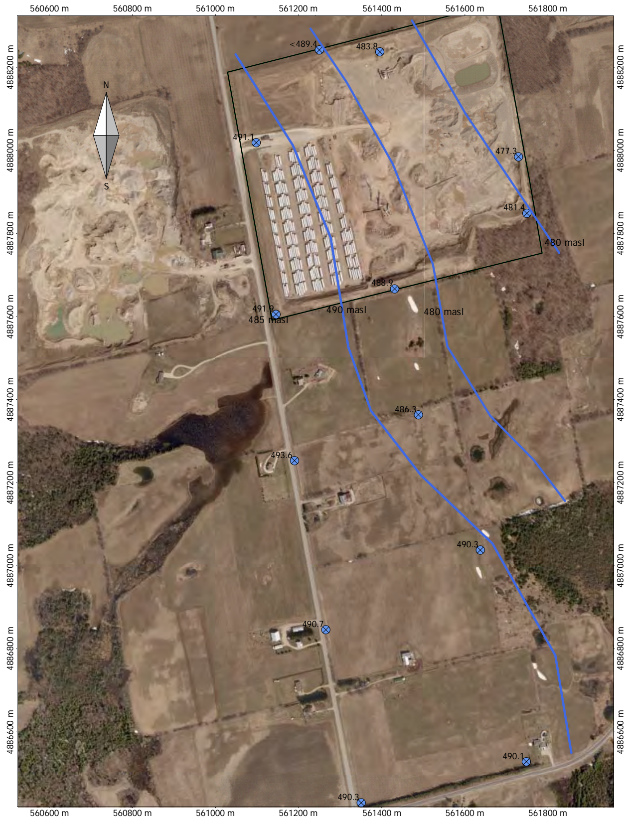
FIGURE 6: BEDROCK GROUNDWATER FLOW CONTOURS
