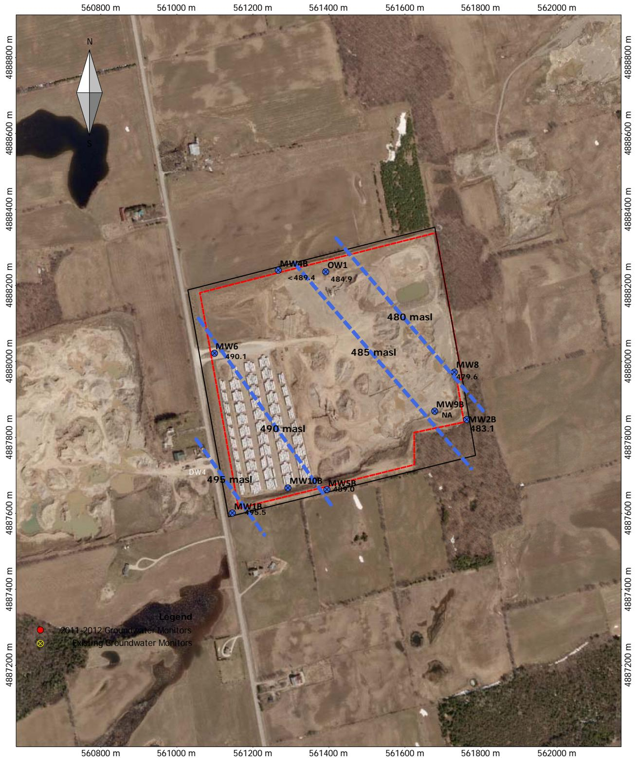
**FIGURE 6: GROUNDWATER FLOW CONTOURS**
